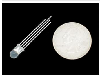
ColorView Components In addition to a processor and a color sensor, you will need an RGB LED (http://adafru.it/159) and some resistors:
