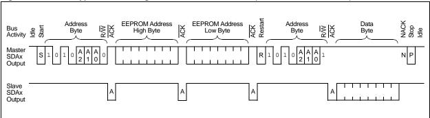
The I<sup>2</sup>C module supports Master mode communication with the inclusion of the Start and Stop generators, data byte transmission, data byte reception, Acknowledge generator and a BRG. Generally, the user software will write to a control register to start a particular step, then wait for an interrupt or poll status to wait for completion. These operations are discussed in the subsequent sections.
