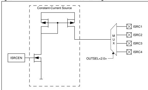
Figure 12-1: Constant-Current Source Module Block Diagram
