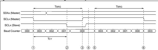
Figure 6-1: Baud Rate Generator Timing with Clock Synchronization
