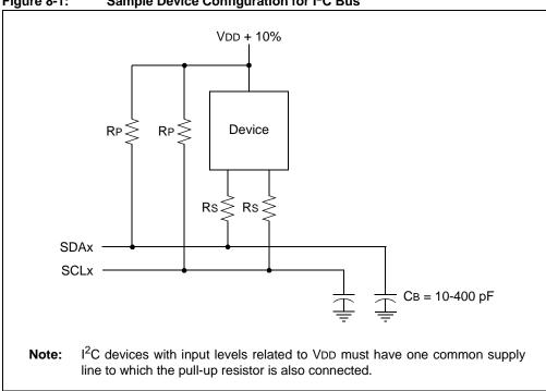
Figure 8-1: Sample Device Configuration for I<sup>2</sup>C Bus
