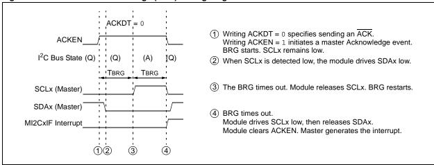
Figure 5-6: Master Not Acknowledge (NACK) Timing Diagram
